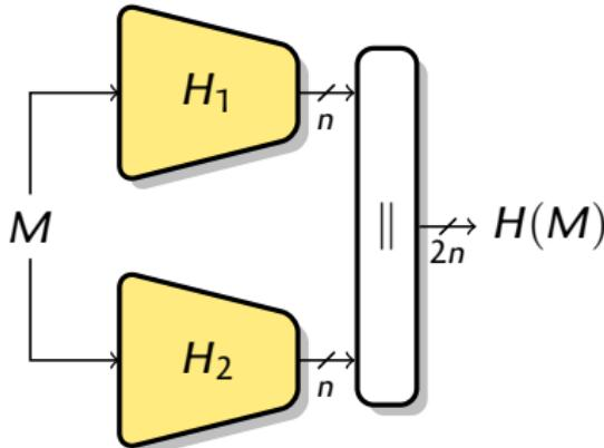
*"In order to make the PRF as secure as possible, it uses two hash algorithms in a way which should guarantee its security if either algorithm remains secure."*
