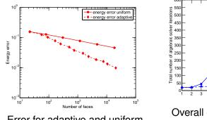
Error for adaptive and uniform mesh refinement
