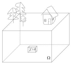
Underground with a water well of f > 0 and pressure head u
