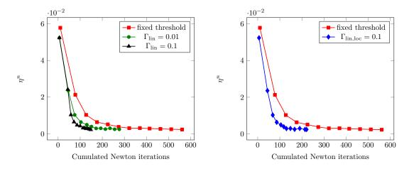
Figure 4: Error estimator  $\eta^n$  (5.2) as a function of the cumulated Newton iterations at each time step (time steps are identified by markers). Global stopping criterion (4.1) (*left*), local stopping criterion (7.4) (*right*)
