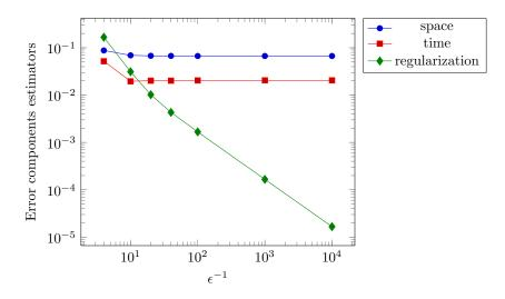
Figure 5: Evolution of the spatial, temporal, and regularization error estimators (3.14) as a function of  $\epsilon^{-1}$  for a fixed mesh and time step
