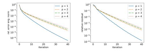
FIG. 9. Nested cubes case: decay of the relative algebraic error (left) and of the relative residual (right) for the hierarchy with  $p_j = 1$ ,  $j \in \{1, \ldots, J-1\}$ , J = 4. The solver of Definition 4.1 is stopped at iteration i = 40. nDoFs: 7281 for p = 1, 55649 for p = 2, 185041 for p = 3, 435393 for p = 4.
