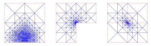
FIG. 5. Graded meshes obtained by the newest-vertex bisection algorithm. Left: Peak problem, J = 10, and p = 3. Center: L-shape problem, J = 10, and p = 3. Right: Checkerboard  $O(10^6)$ , J = 10, and p = 3. The regions where the diffusion coefficient is constant are bordered by dashed lines.
