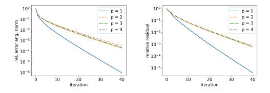
FIG. 8. Cube case: decay of the relative algebraic error (left) and of the relative residual (right) for the hierarchy with  $p_j = 1$ ,  $j \in \{1, \ldots, J-1\}$ , J = 4. The solver of Definition 4.1 is stopped at iteration i = 40. nDoFs: 5501 for p = 1, 41337 for p = 2, 136693 for p = 3, 320753 for p = 4.
