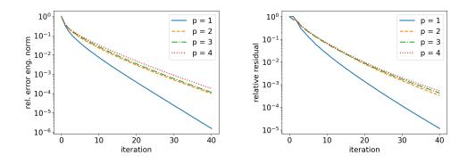
FIG. 10. Checkers cubes: decay of the relative algebraic error (left) and of the relative residual (right) for the hierarchy with  $p_j = 1$ ,  $j \in \{1, \ldots, J-1\}$ , J = 4. The solver of Definition 4.1 is stopped at iteration i = 40. nDoFs: 5425 for p = 1, 40033 for p = 2, 131473 for p = 3, 307393 for p = 4.
