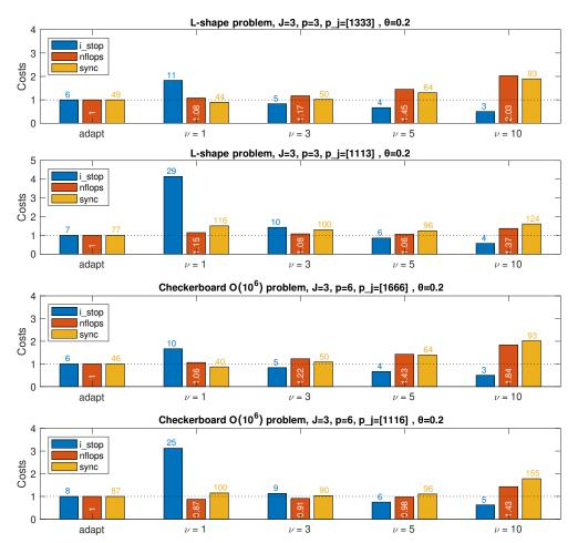
FIG. 7. Comparison between a fixed number of (block-Jacobi) smoothing steps  $\nu$  on all levels (Definition 4.1 and its obvious modification for  $\nu \geq 1$ ) and the adaptive number of smoothing steps of Definition 7.1. Number of iterations  $i_s$ , floating point operations given by (8.1) relative with respect to Definition 7.1, and the number of global synchronizations by (9.6).
