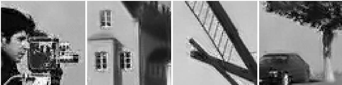
Figure 10.2 – Illustration of the noise halo appearing around high contrasted edges on images denoised by the NLM. The input noisy images are corrupted versions of the noise-free images presented on Fig. 10.6 damaged by AWGN with standard deviation \sigma = 20 . Noise halo arises from an abrupt lack of redundancy around edges sometimes referred as the rare patch effect.
