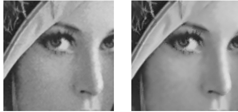
Figure 8.9 – Left and right: extract of the result of the NLM filter with s^2 = 3 \times 3 and s^2 = 5 \times 5 on a noisy image ( \sigma = 10 , h optimized for PSNR). Using a too small patch size makes the algorithm less robust to noise and Lena's skin looks mottled. It looks smoother with patch size 5 \times 5 but visual artifacts appear in the eye.
