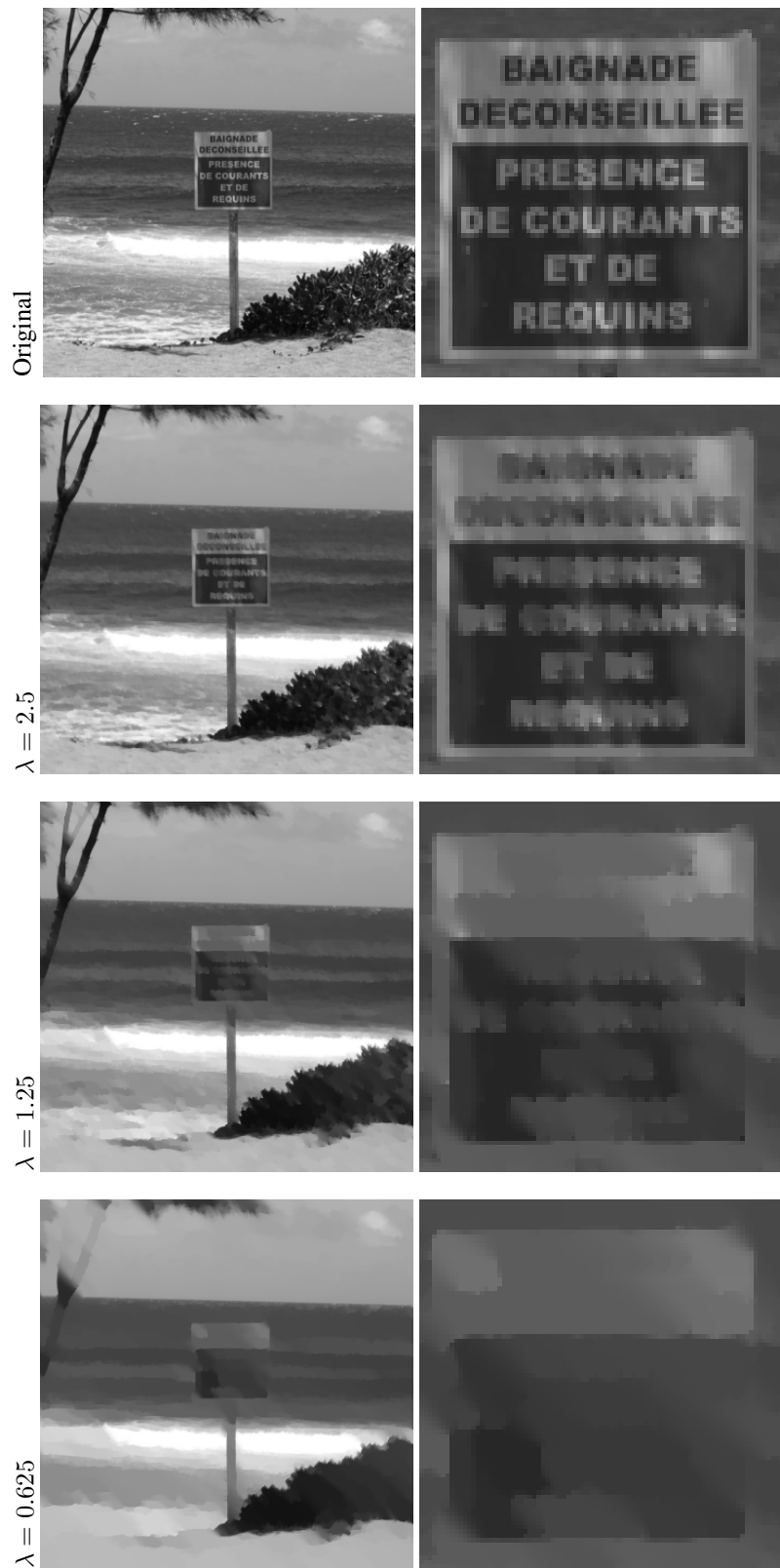
Figure 7.2 – Result of the Pock-Chambolle algorithm [Chambolle and Pock, 2011] with 8-connectivity. As \lambda decreases the Wulff shape appears: it is a rectangle as in 7.1.
