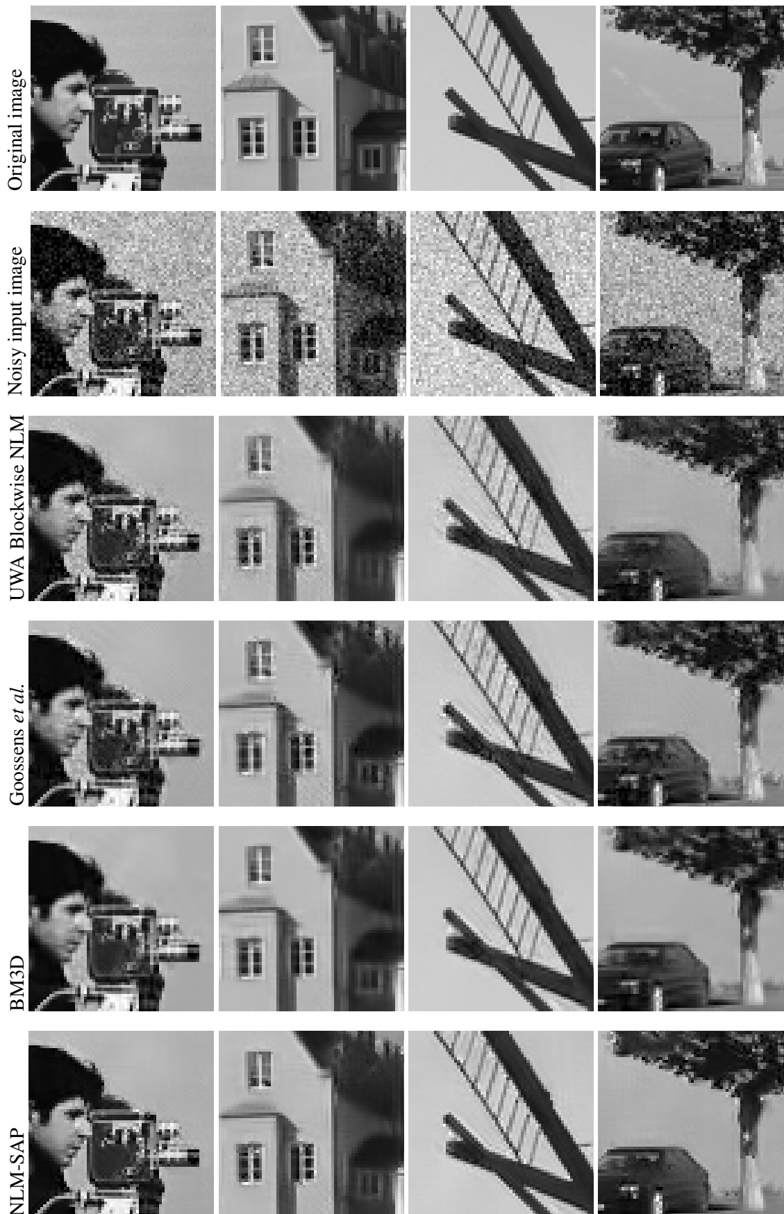
Figure 10.12 – Comparisons of the visual denoising performance of the proposed NLM-SAP and other state-of-the-art methods ( \sigma = 20 ). From top to bottom, the original and noisy images, the results obtained by the classical (pixelwise) NLM [Buades et al., 2005], the blockwise NLM using UWA reprojection for square patches the BM3D denoiser [Dabov et al., 2007], and the proposed NLM-SAP.
