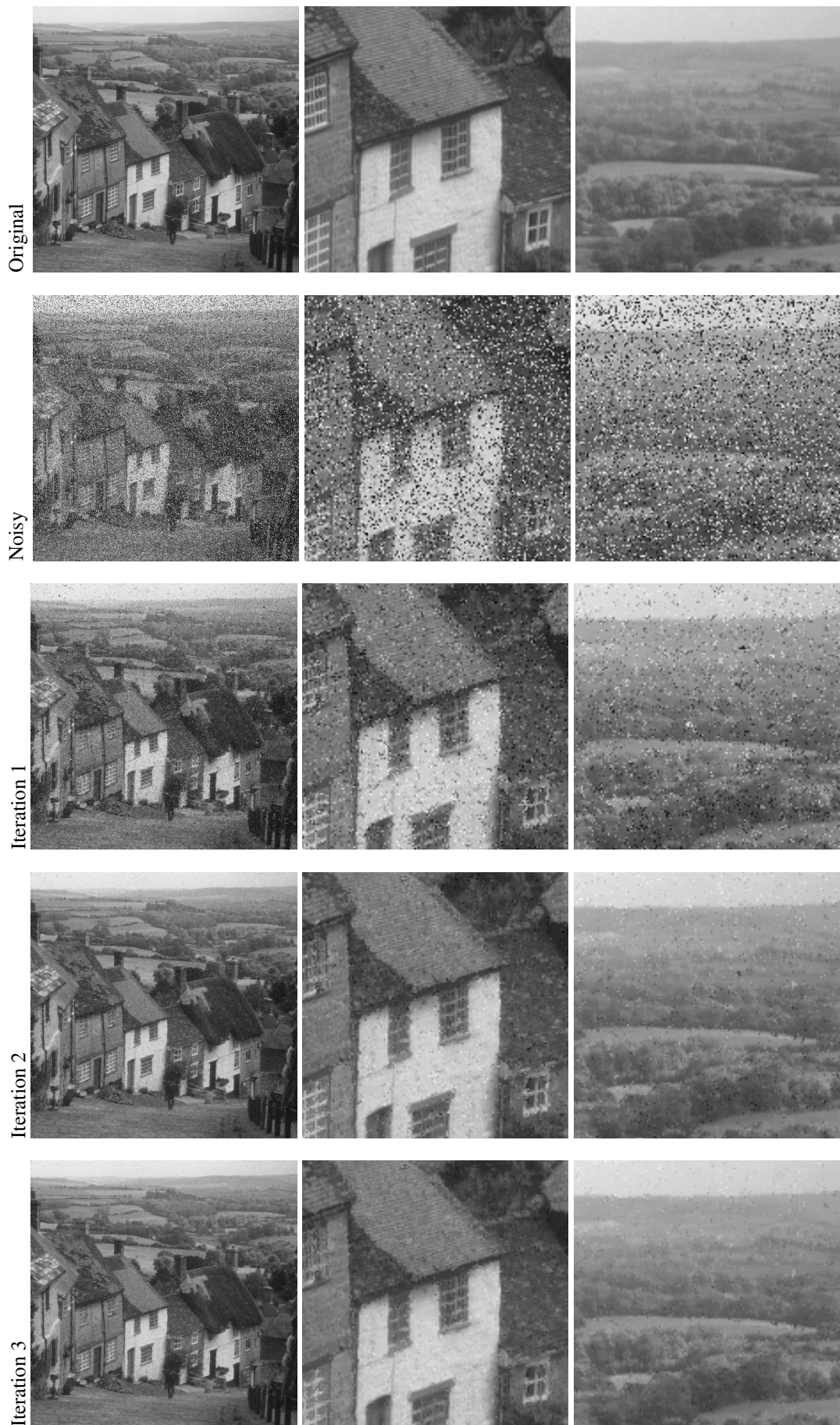
Figure 6.7 – Evolution of the result with the iterations using ROAD-TVLI. The PSNR for iterations 1,2,3 is 21.80 dB, 27.97 dB, 29.75 dB.
