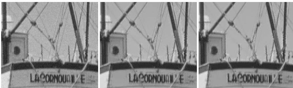
Figure 8.4 – Loss of lines and isolated details. Left: Boat image with little noise ( \sigma = 5 ). Middle: Result of the NLM filter ( h = 6 , s^2 = 7 \times 7 , search window 11 \times 11 ). Right: same experiment, using a search window 61 \times 61 . Notice that several ropes vanish when the size of the search window increases (this should be seen on a computer screen).
