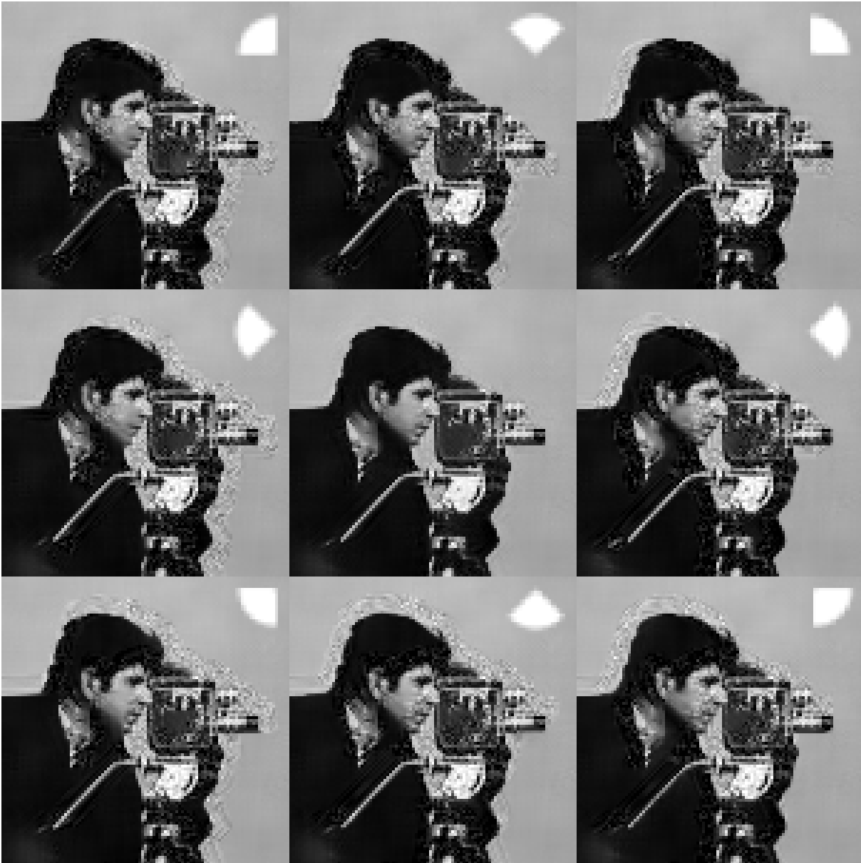
Figure 10.8 – Eight denoised images obtained for different oriented patch shapes. The proposed final aggregate is in the center. Each denoiser provides good performances in a specific target direction but suffers from noise halos in the other directions. The final (central) aggregate takes advantage of every oriented-denoiser to provide high quality restored edges. The patch shape used is indicated in white.
